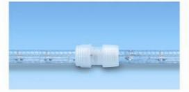
5.Install the End Cap (WW-FLS-2W-ER-A) and inject the waterproof material to complete the waterproof function.
